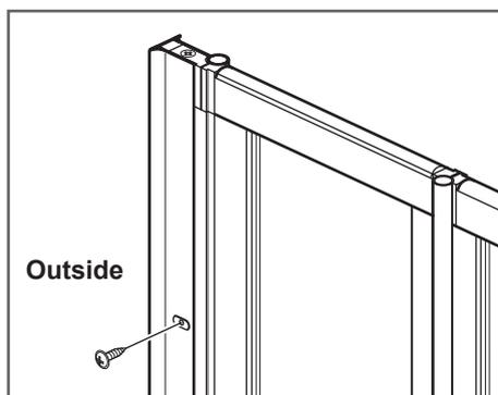
Remove the 2 screws from the side of the wall channel (keep them safe) and remove the wall channel from the bath screen.
