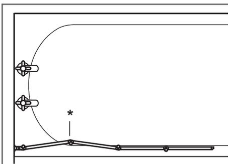
When in use the panel nearest the wall should be angled in as shown (\*).
