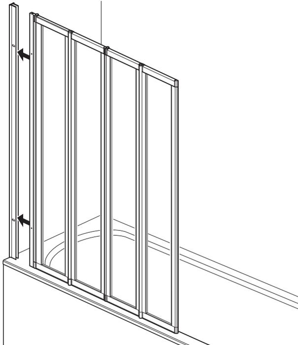
With help, push the bath screen into the wall channel. Align the holes in the bath screen with the slotted holes in the wall channel, fix securely in position using the 2 screws removed in step 2. The slotted holes in the wall channel allow the screen to be adjusted until it is level and the bottom of the water seal makes even contact along the bath rim and still allows it to move as required.
