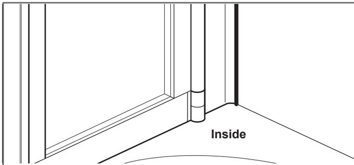
**Sealing:** On the inside and outside, run a line of silicone sealant from top to bottom down the joint between the wall channel and tiles.
