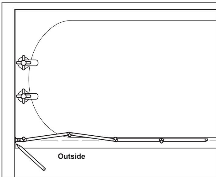
The bath screen should be positioned on the inner edge of the bath rim, as shown.
