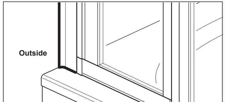
**Outside only:** Run a line of silicone sealant along the joint between the bottom edge of the wall channel/hinge stile and bath rim as shown.
