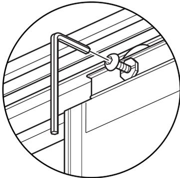
**If the doors are not square with the fixed panels or they don't close correctly, one or both of the top sliders should be adjusted.**
