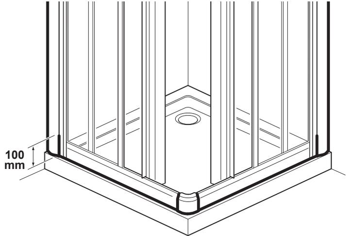
**Sealing outside:** Run a line of silicone sealant from top to bottom down the joint between the wall channels and tiles. Run a line of silicone sealant 100mm up the joint where the side panels slot into the wall channels. Run a line of sealant around the base in the joint between the bottom of the enclosure and the tray, from wall to wall.
