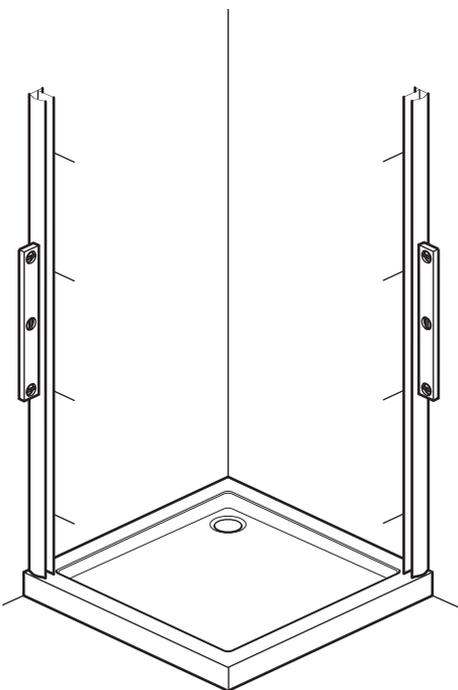
Remove both wall channels from each side of the enclosure. Place each wall channel in position on the tray (10 - 15mm in from the outer edges of the tray), use a spirit level to ensure they are vertical and mark all 8 fixing holes onto the walls (holes inside).
