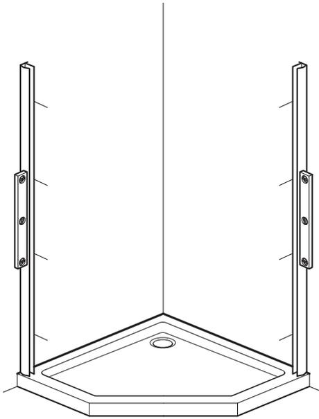
Remove both wall channels from the door frame. Place each wall channel in position on the tray (10 - 15mm in from the outer edges of the tray), use a spirit level to ensure they are vertical and mark all 8 fixing holes onto the walls (holes inside).
