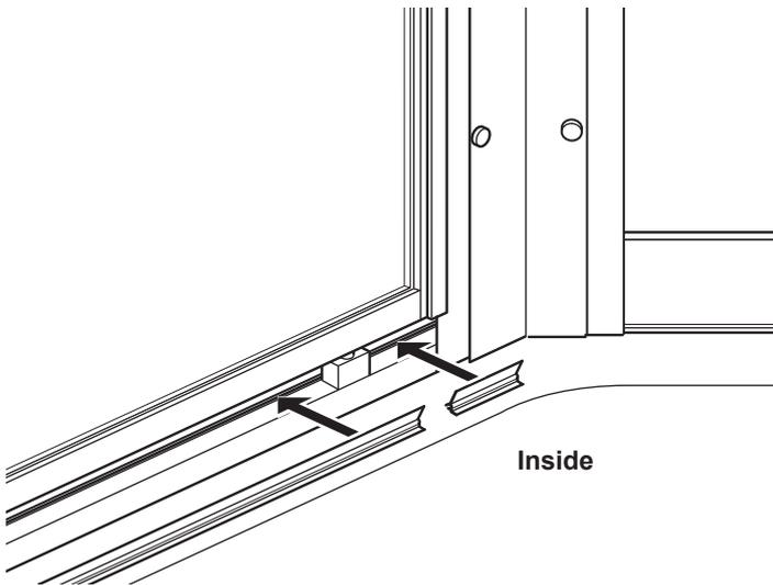
**Optional:** It is only necessary to fit the plastic Anti splash strip (E) if water splashes out through the gap under the door. Cut the strip to size (using scissors) and push fit onto the lug shown on the bottom door frame as shown.
