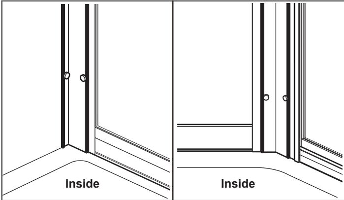
**Sealing inside:** Run a line of silicone sealant from top to bottom down the joint between the wall channels and tiles. Run a line of silicone sealant from top to bottom down the joint where the pent panels slot into the wall channels and the pent panels and door slot into the pent posts.
