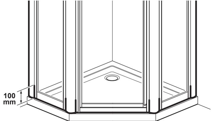
**Sealing outside:** Run a line of silicone sealant from top to bottom down the joint between the wall channels and tiles. Run a line of silicone sealant 100mm up the joint where the pent panels slot into the wall channels and pent posts. Run a line of sealant around the base in the joint between the bottom of the enclosure and the tray, from wall to wall.
