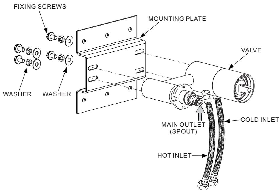
**FIG. 1 INSTALLATION OF SPOUT**
