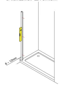
Remove wall channel from the glass panel frame. Place wall channel in position on the tray (8 - 12mm in from the outer edge of the tray), use a spirit level to ensure that they are vertical and mark all 3 fixing holes onto the wall.
