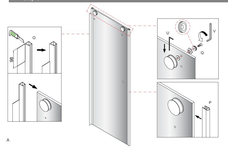
Hung the glass door to the top track, at the bottom make the glass door into the slot of the glass clamps (M). Slide the roller 2 to align with the fixing hole of glass door, Insert the washer from the roller 2 connector (R) between the roller 2 and the glass door. Stop the roller 2 moving using the allen key (V).
