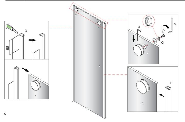
Hung the glass door to the top track, at the bottom make the glass door into the slot of the glass clamps (M). Slide the roller 2 to align with the fixing hole of glass door, Insert the washer from the roller 2 connector (R) between the roller 2 and the glass door. Stop the roller 2 moving using the allen key (U) to fix roller 2 connector (R) to the glass door using the allen key (V).
